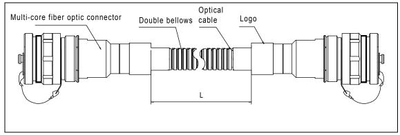
Features: Both ends of the optical cable are multi-core optical fiber cable connectors. The optical cable is an indoor optical cable and is protected by a double-layer corrugated pipe.
